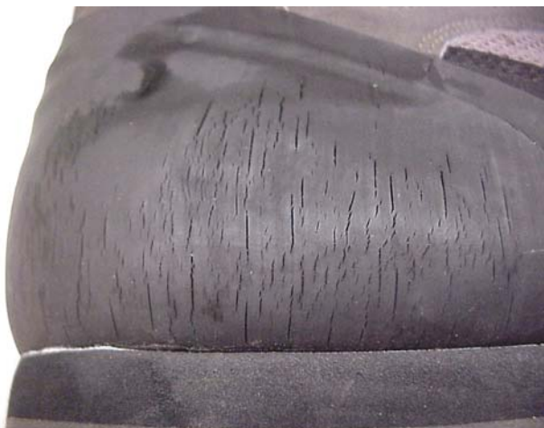
Figure 7. Wader boot exposed to benzethonium chloride had cracking of rubber toe.
